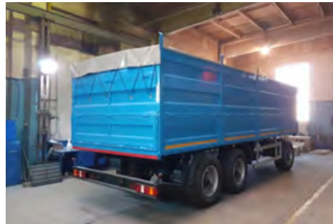
Three-axis sided grain trailer Transported cargo 33 m2
