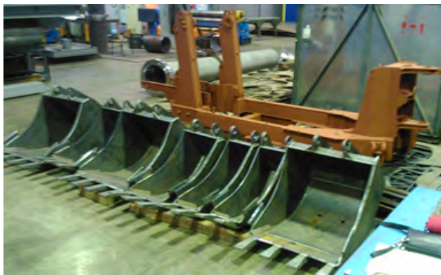
Spare parts for EO-2621 and EO-2626 excavators based on MTZ/UMZ tractors
