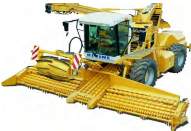
RL 200 self-propelled beet loading-and-cleaning harvester
