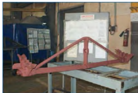
Transversal brake bar for freight-car trucks of main railway lines
