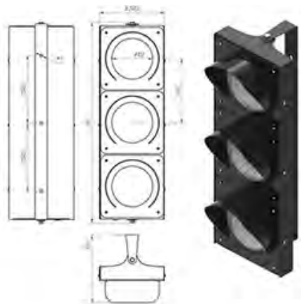
LED traffic lights -single-section 100 mm SS1 -two-section 100 mm SS2 -three-section 100 mm SS3 Multipurpose light traffic sign
