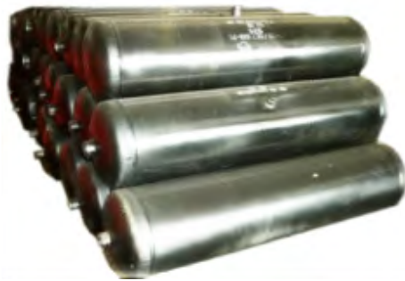
Air reservoirs for railway air brake system
