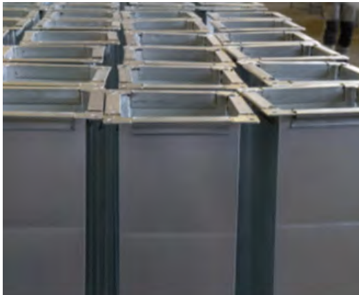
Rectangular air ducts
